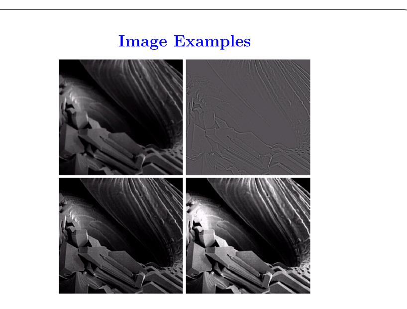
Top-left: original, top-right: laplacian, bottom-left: laplacian and original, bottom-right: laplacian and original with A > 1, boosted
