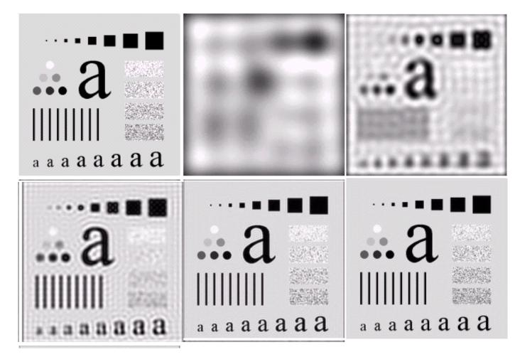
Low pass filtering with different cutoff frequencies. Top-left original, others filtered with 8, 5.4, 3.6, 2.0, 0.5 percentage removed
