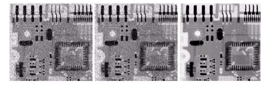
Left: image corrupted by salt pepper noise, middle: linear smoothing filtering, right: median filtering
