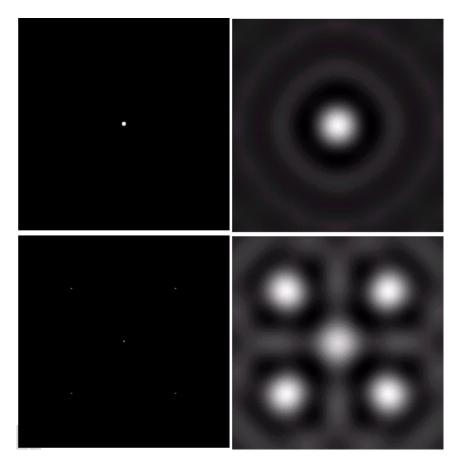
Top-left: ideal low pass filter in the frequency domain, top right: ideal low pass filter in spatial domain, bottom-left: test image, 5 impulses, bottom-right: filtered version of the test image
