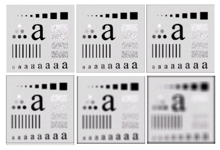
Top-left: original, from top to bottom and left to right: linear smoothing with increasing filter size
