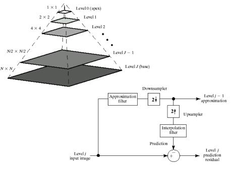
Left: Image pyramid, right: block diagram for one level
